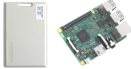
(a) Bluetooth Beacon [15] (b) Raspberry Pi 3 SBC [16]
